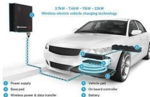
Static Wireless Charging Station (SWCS)
